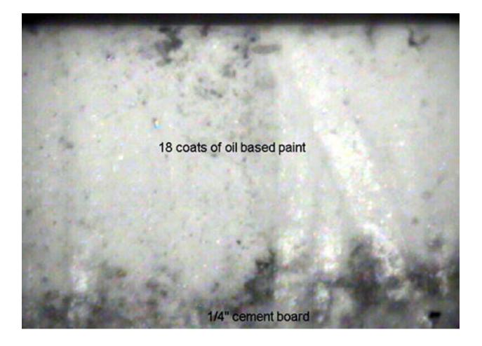
1/4" Cement Board with 18 coats of oil based paint and 8-10 wet mils of Rust Grip
