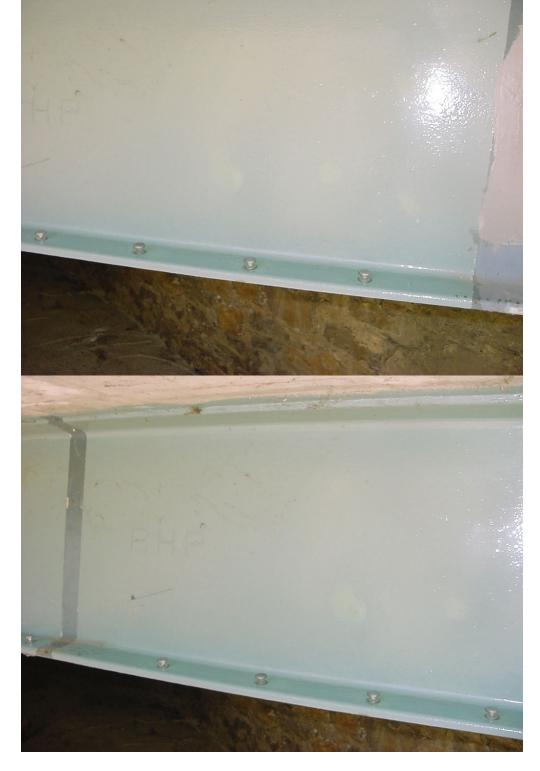
Round spots mark the area where pull dollies were attached to perform pull tests.
