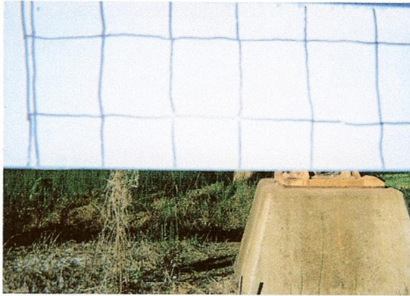
ASTM 610 Rust grade 9 M 714 Scale 10
