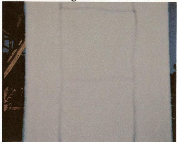
ASTM 610 Rust grade 10 M 714 Scale 10
