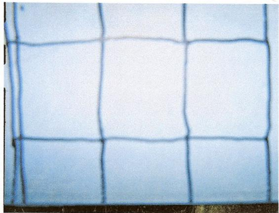
ASTM 610 Rust grade 9 M 714 Scale 10
