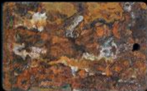
Naval Jelly® Rust Neutralizer Topcoated with Napa Ruf-Nek HD Spray Paint
