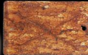
Zinc-Chromate Primer Topcoated with Zynolyte Urethane
