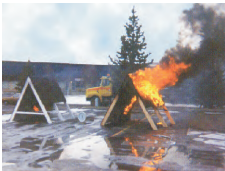
SafeCoat coated interior roof space and an untreated roof space under identical fire conditions
