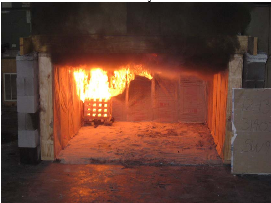
Calibration test. Flames out the front.
